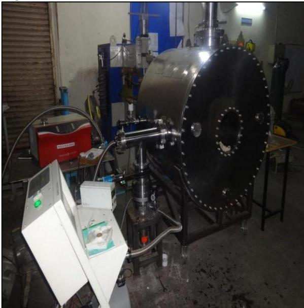
Vacuum leak test setup
