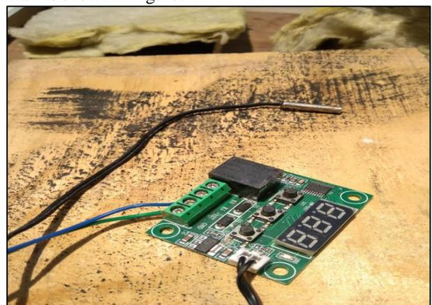
Fig. 5: Temperature sensor with digital indicator
