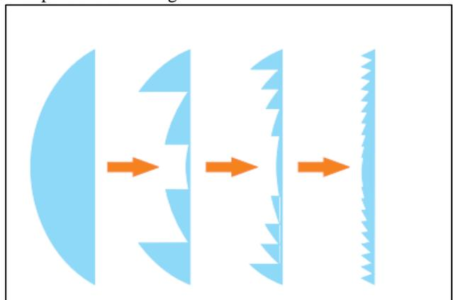
Fig. 2: Collapsing a continuous surface aspheric lens into an equivalent power fresnel lens.
