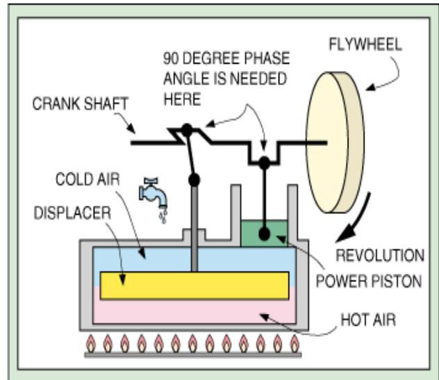
Fig. 1: Gamma type Stirling engine
