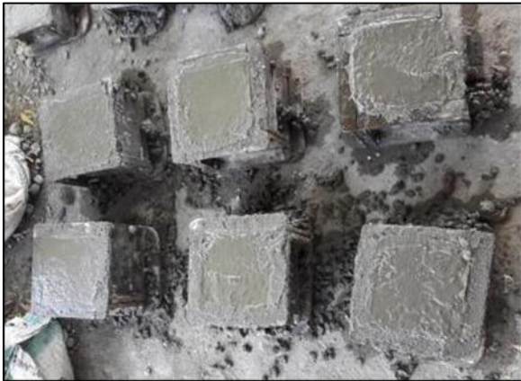
Fig. 4: Concrete Mix With 10% ESP as Partial Replacement for Cement
