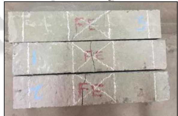
Fig. 7: Prism after Failure
