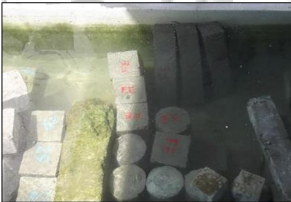
Fig. 6: Curing Of Specimen
