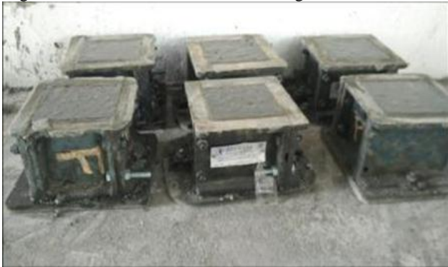
Fig. 3: Concrete filled moulds
