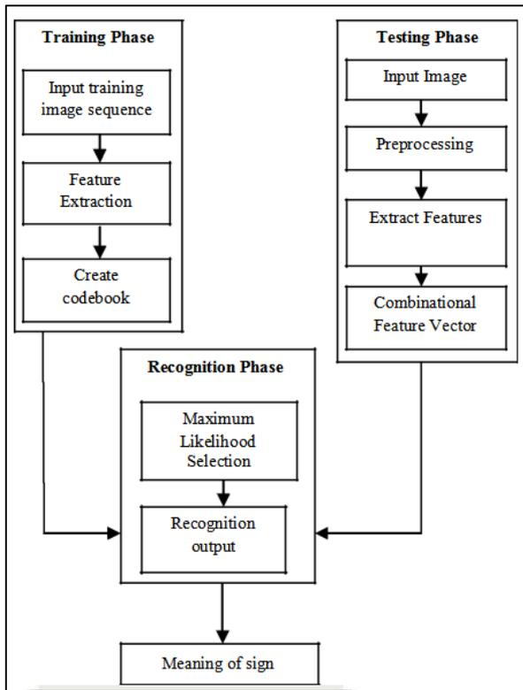
Fig. 2: Block diagram of hand gesture recognition system
