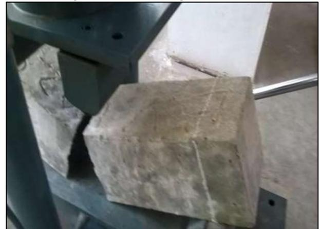
Fig. 5: Flexural Strength Test
