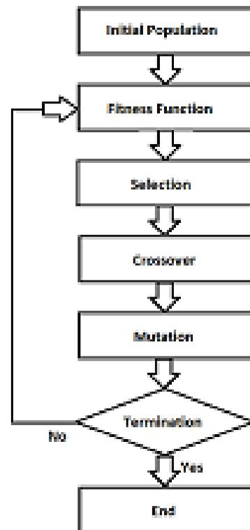
Fig. 4: Genetic Algorithm architecture.
