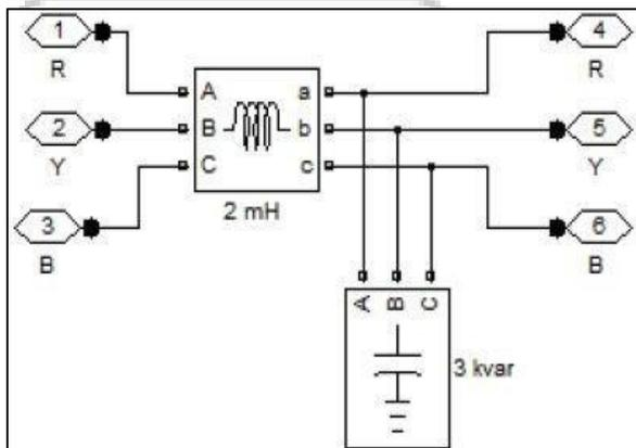
Fig. 2: Filter implementation on MATLAB Simulink.
