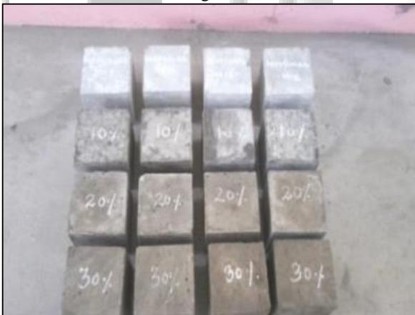
Fig. 3: Replacing the cement with Lime sludge waste in cube.
