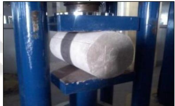
Fig. 5: Tensile strength of Lime sludge waste in 28 days
