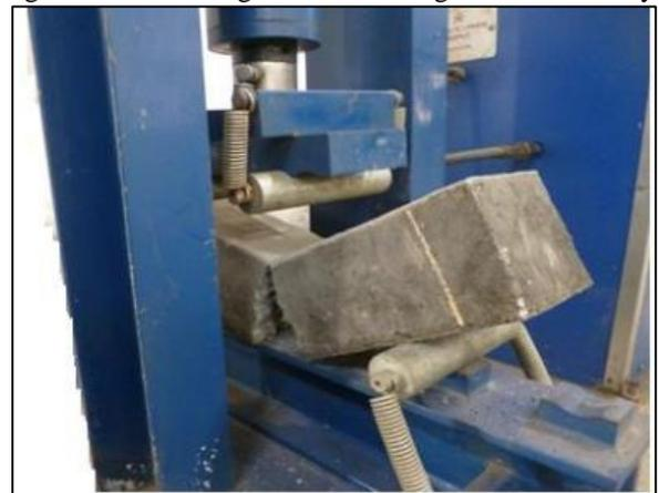
Fig. 6: Flexural strength of Lime sludge waste in 28 day
