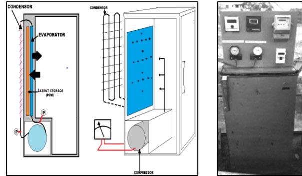
Fig. 1: (a) 3D model of test facility (b) Actual model
