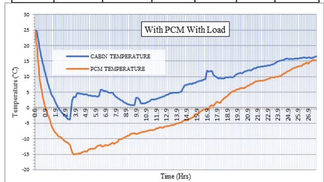
Fig. 3: Temperature v/s Time (With PCM with Load Condition)
