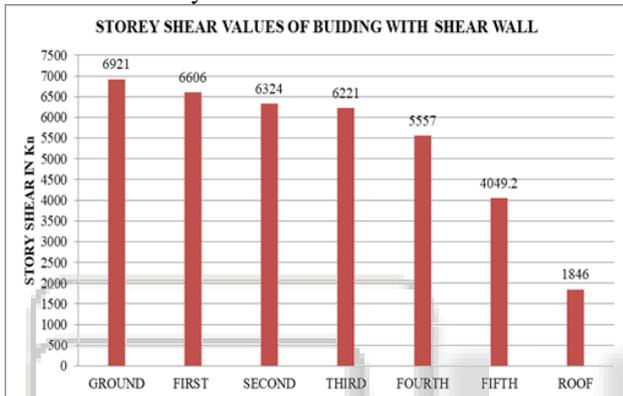
Fig. 6: Storey shears of the model with Shear wall
