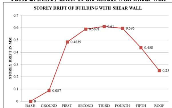
Fig. 5: Storey drifts of the model with Shear wall
