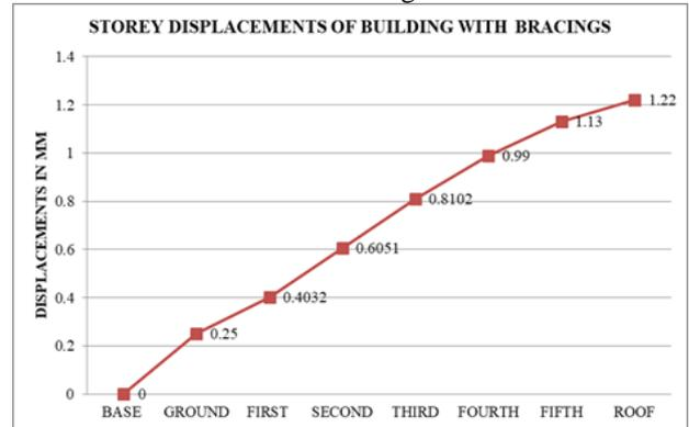
Fig. 8: Storey displacements of the model with Shear wall and Bracings.
