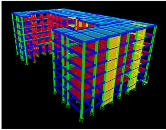
Fig. 1: Shear wall assigned to the building.
