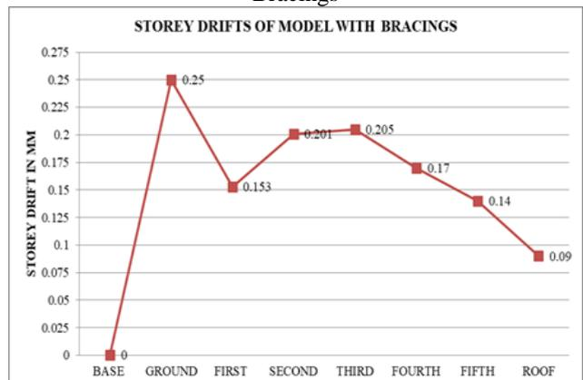
Fig. 9: Storey drifts of the model with Shear-wall and bracings.
