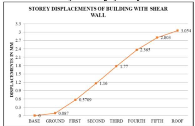
Fig. 4: Storey displacements of the model with Shear wall
