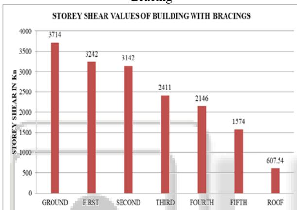
Fig. 10: Storey shears of the model with Shear wall and Bracings.
