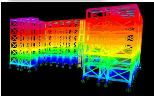
Fig. 7: Deflection due to dynamic FNA with Bracings.
