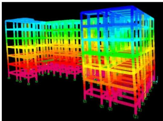
Fig. 3: Deflection due to dynamic FNA with Shear wall.
