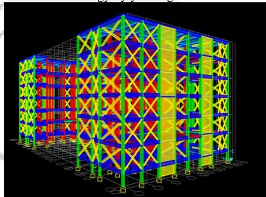
Fig. 2: Bracings assigned to the building.
