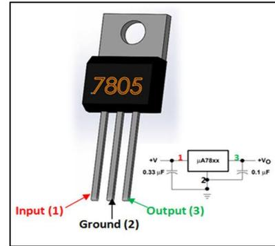
Fig. 6: Voltage Regulator (IC-7805)
