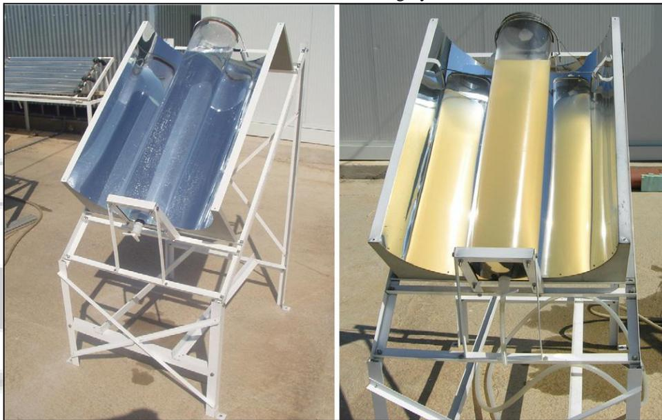
Fig. 2. SODIS enhanced batch reactor of 25 L containing water of 0 and 100 NTU
