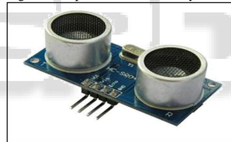
Fig. 2d: Ultrasonic Sensor
