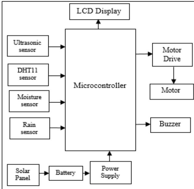
Fig. 1: Block Diagram of Solar Power Auto Irrigation System
