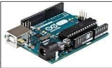
Fig. 2: Arduino UNO development board
