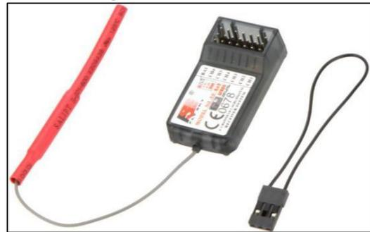
Fig. 9: Receiver of CT 6B Transmitter
