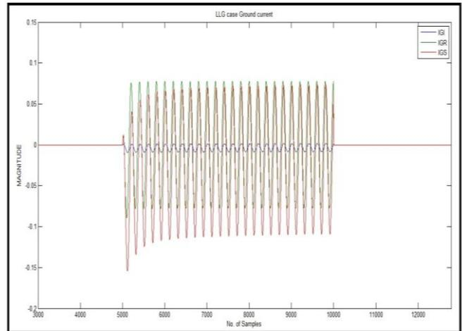
Fig. 4: Time domain waveform of LL-G fault for all Groundings
