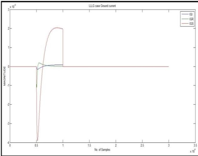
Fig. 6: Time domain waveform of LLL-G fault for all Groundings
