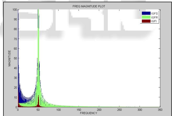
Fig. 5: Frequency domain waveform of LL-G fault for all groundings
