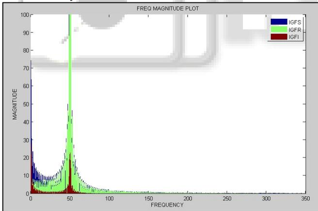
Fig. 3: Frequency domain waveform of L-G fault for all groundings
