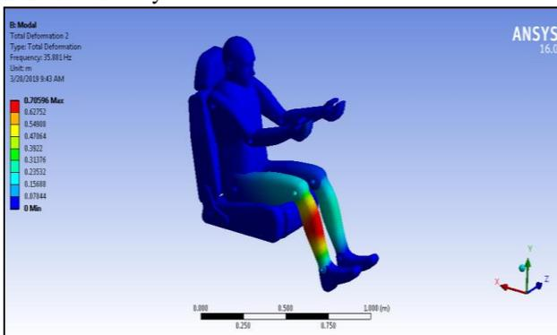
Fig. 2: Mode shape of 76 kg human subject at natural frequency 35.881 Hz
