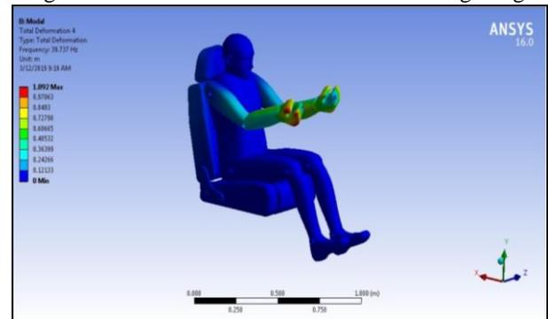
Fig. 4: Mode shape of 76 kg human subject at natural frequency 39.737 Hz
