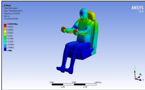
Fig. 1: Mode shape of 76 kg human subject at natural frequency 22.118 Hz
