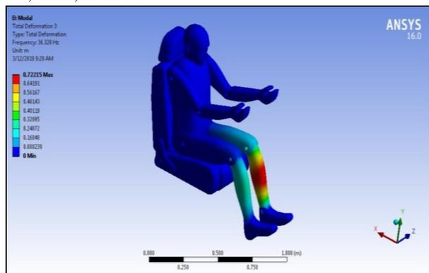
Fig. 3: Mode shape of 76 kg human subject at natural frequency 36.328 Hz
