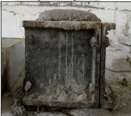
Fig. 3: Casting of Cube
