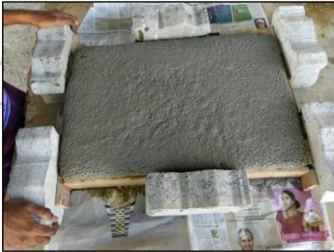
Fig. 2: Casting of Slab
