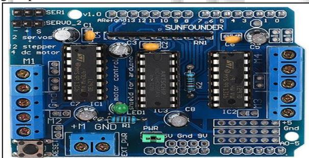
This motor driver expansion board is based on the L293D chip which is designed to drive up to 4 bidirectional DC motors with individual 8-bit speed selection. It can also drive 2 stepper motors (unipolar or bipolar), single coil or double coil, interleaved or micro-stepping. It contains 4 H-bridges which provide up to 0.6 A per bridge (1.2A peak) at voltages from 4.5 V to 36 V.
