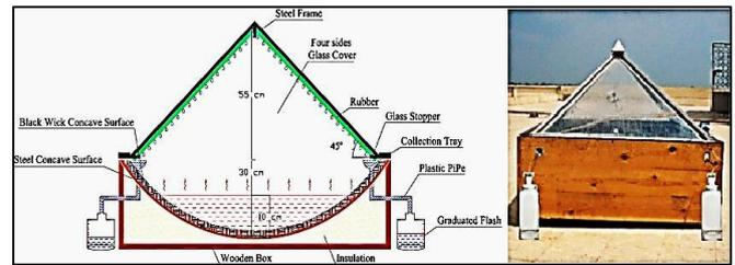
Fig. 11: Concave type solar still; (a) schematic diagram (b) experimental setup
