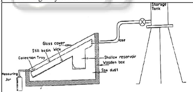
Fig. 10: Schematic representation of wick type solar still
