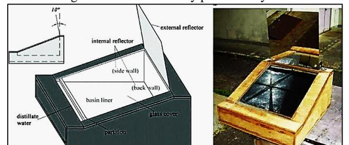
Fig. 5: Single slope still with internal and external reflectors; (a) schematic (b) experimental setup
