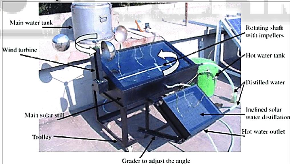
Fig. 8: Single slope still using rotating shaft
