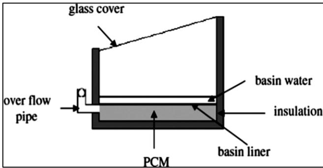
Fig. 9: Schematic diagram of the single slope-single basin solar still with PCM
