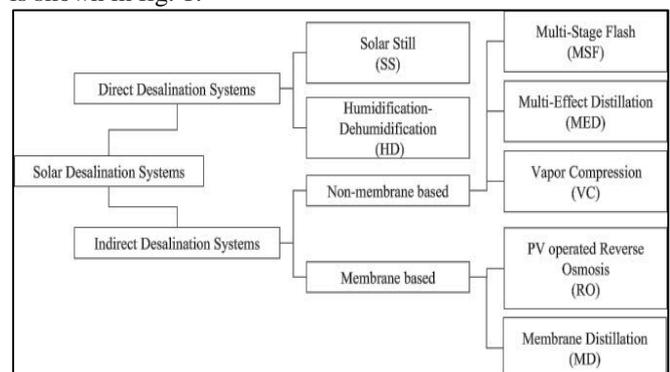
Fig. 1: Classification of solar desalination systems
