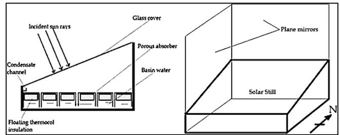
Fig. 7: Single slope still with porous absorber on the thermocol insulation
