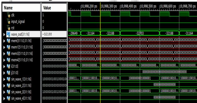
Fig. 7: HDL Simulation waveform for QAM.
