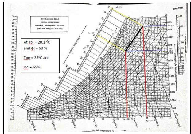
Analysis of psychrometric chart for: Sample calculation Silica gel and CaCl<sub>2</sub>
