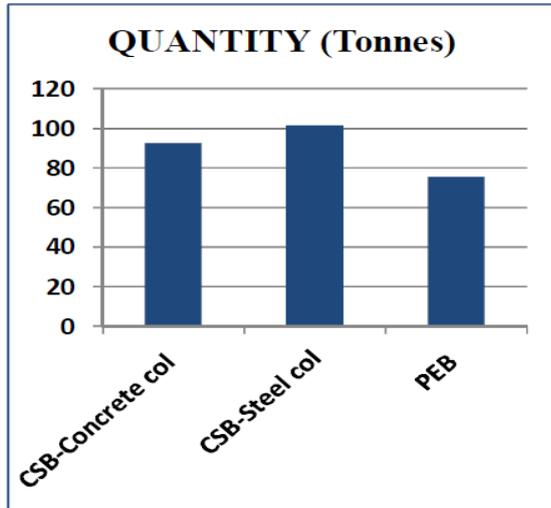
Figure 8: Quantity of Steel Utilized For the Structure
