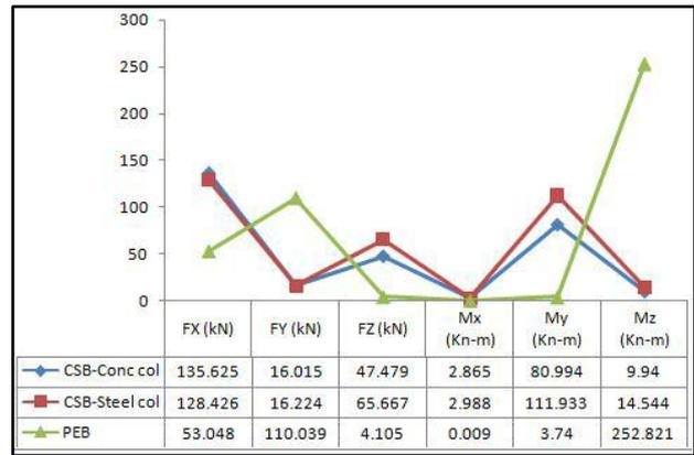
Figure 5: Bending moments and Reactions in Rafters
