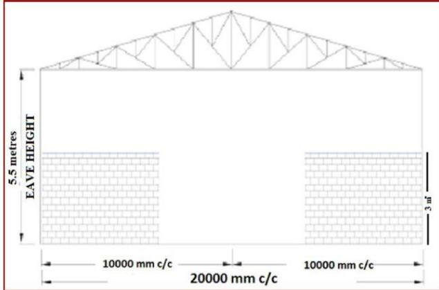
Fig.2 Single Frame of a Conventional Steel Building
