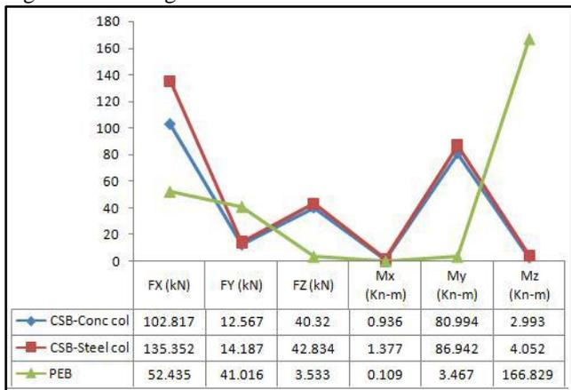
Figure 8: Bending moments and Reactions at Ridge Portion
