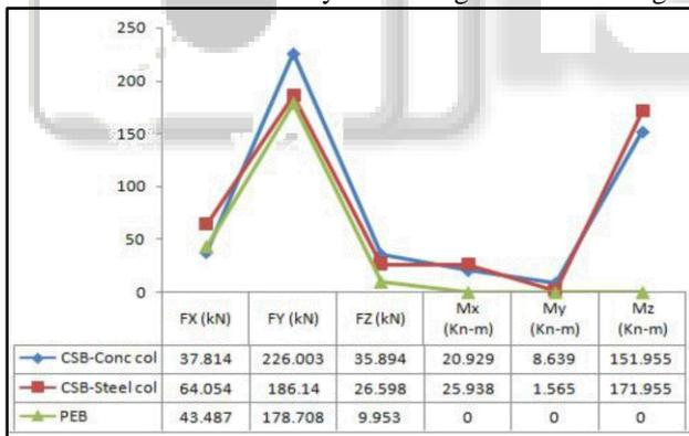
Figure 3: Bending moments and Reactions at Supports
