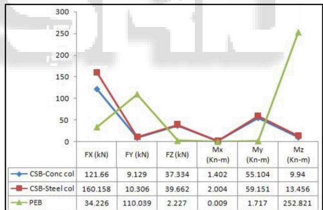
Figure 7: Bending moments and Reactions at end of Rafters
