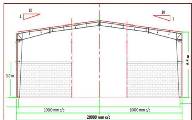
Fig.1 Single Frame of a Pre Engineered Building
