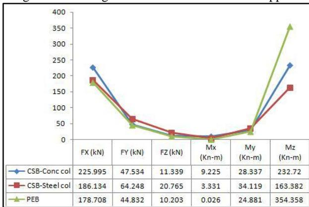
Figure 4: Bending moments and Reactions in Columns
