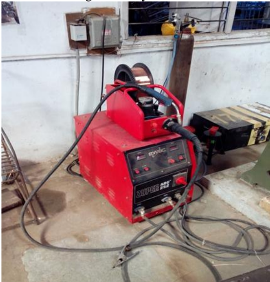
Fig. 4.1: MIG welding machine [22]
