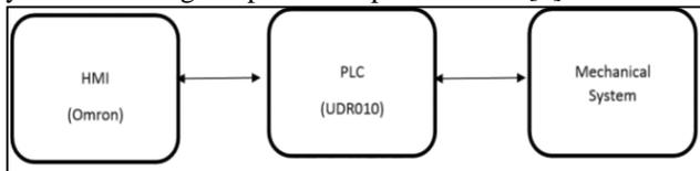
Fig. 1: Connections between the peripherals, PLC and HMI (display). The basic components in a ladder logic program are the contact and the coil. The contact is the name given to a general input device set by an external switch, an internally set logic or timer function. Coil is the name given to an output device and is used to drive relays, contactor, motors, solenoids and other process actuators [8].
