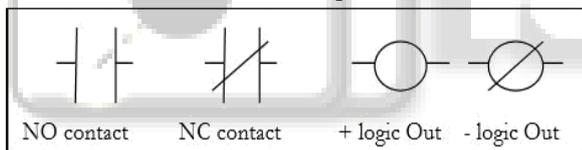
Fig. 2: Basic Ladder Logic Components.
