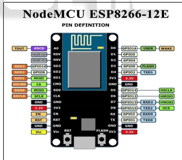
Fig. 1: ESP8266 Microcontroller
