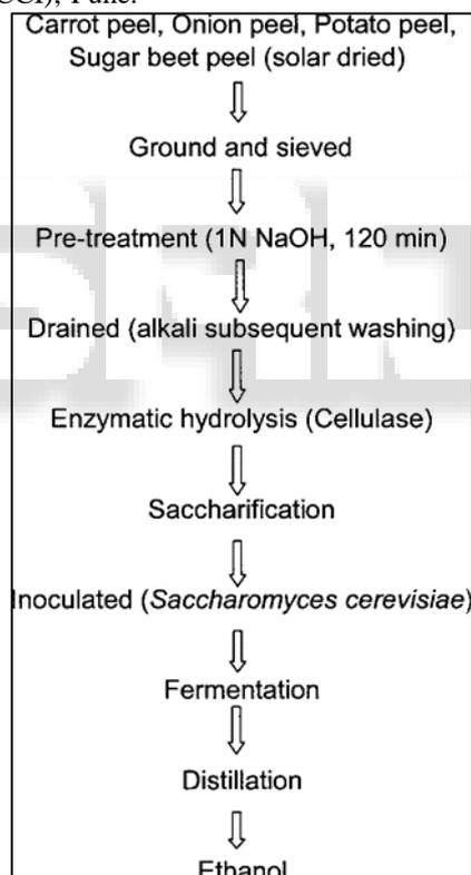
Fig. 1: Flow diagram for production of ethanol using cellulase enzyme
