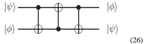
Fig. 6: Swap Gate Using Three CNOT Gate
