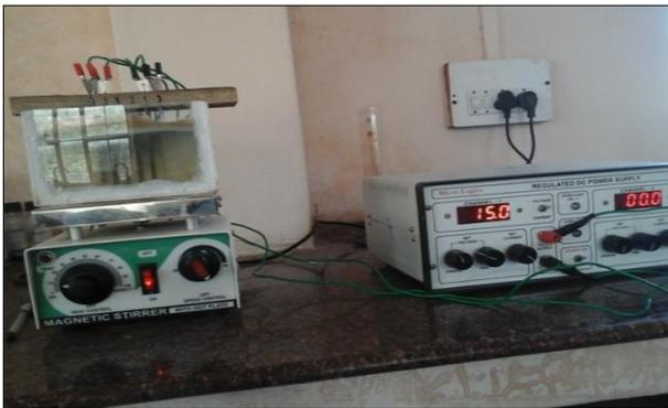
Schematic connections for Electrodialysis process
