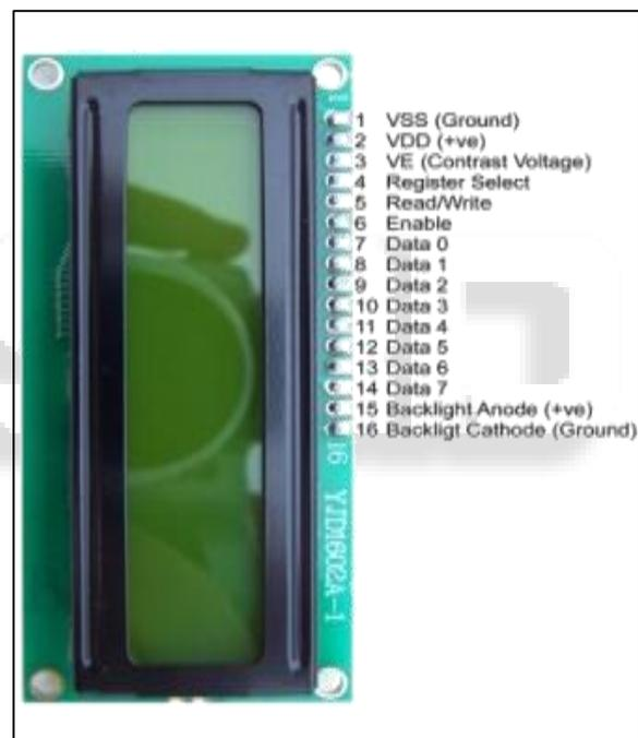
Fig. 7: LCD Display
