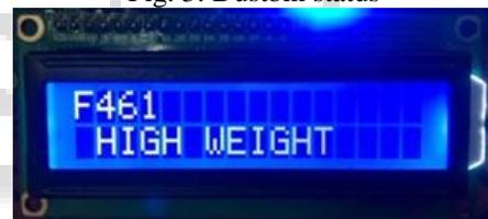
Fig. 4: Dustbin Status when threshold limit exceeds
