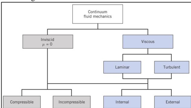
Fig. 1.1: Basic components of fluid mechanics
