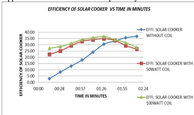
Fig. 3: Variation efficiency of solar cooker and time taken to efficiency of solar cooker
