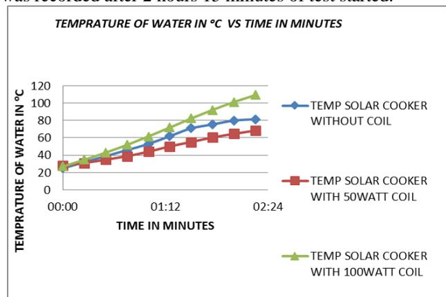
Fig. 2: Variation of water temperature and time taken to reach the water temperature
