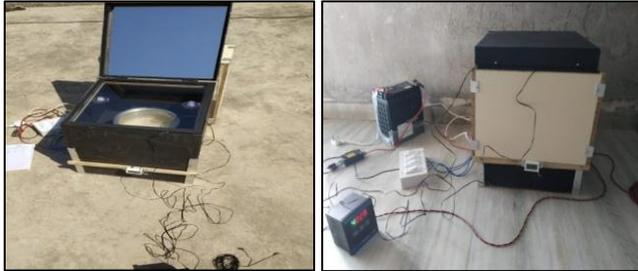
Fig. 1: (A) Experimental setup of fabricated solar cooker with measuring instruments, (B) Experimental set up with coil arrangements with battery and measuring instruments
