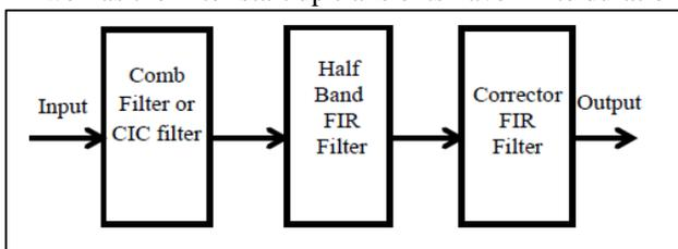
Fig. 2: Block diagram of decimation filter
