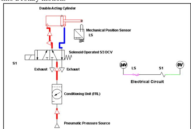
Fig. 1: DAC Solenoid Valve Circuit Diagram
