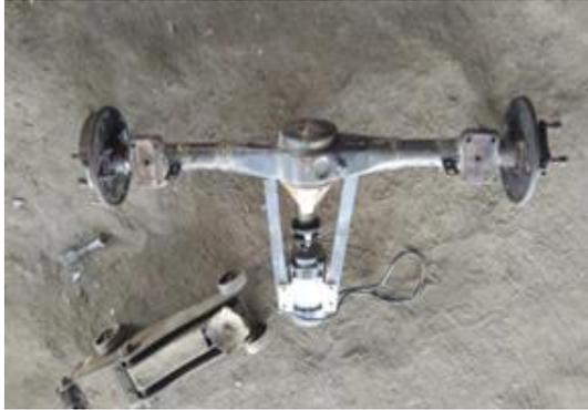
We replaced the rear axle of Maruti with the rear axle of omni due to the same width of the axle. We added a two base plates by gas welding to give support for the suspension system of the vehicle.
