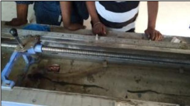
Fig. 2: deformation of blended bitumen
