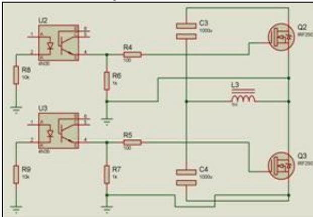
Fig. 2: (b) Decoupling circuit
