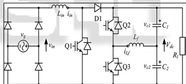
Fig. 1: (a) Symmetric half Bridge circuit
