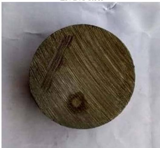
Fig. 5.1: Work piece material: EN-24 tool steel (40 mm diameter)
