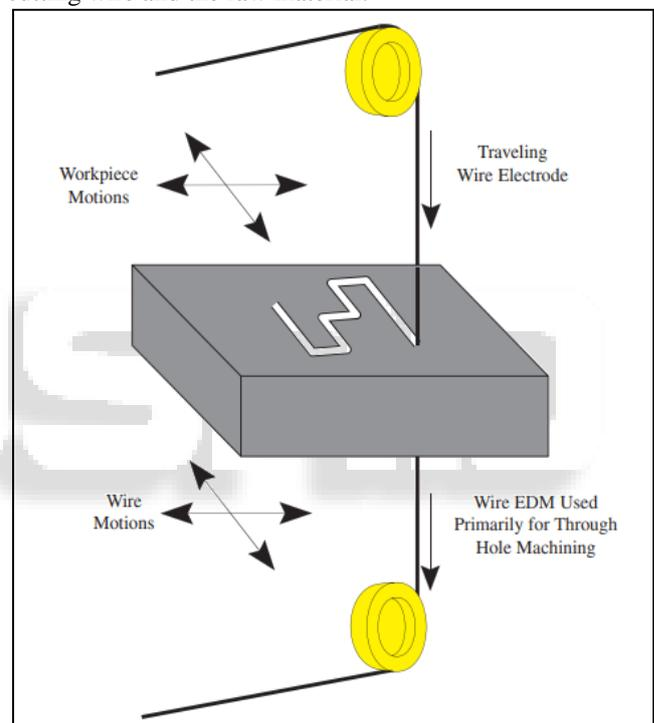
Fig. 2.1: Diagram of working of WEDM
