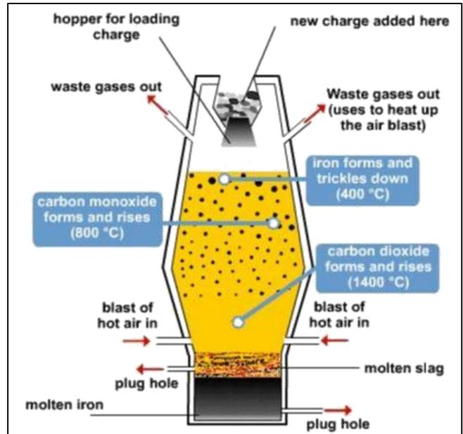
Manufacture and Constituents of Blast-furnace Slag
