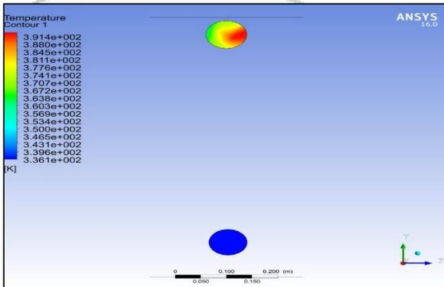
Fig. 5: Temperature of feed water at inlet and outlet of pipe
