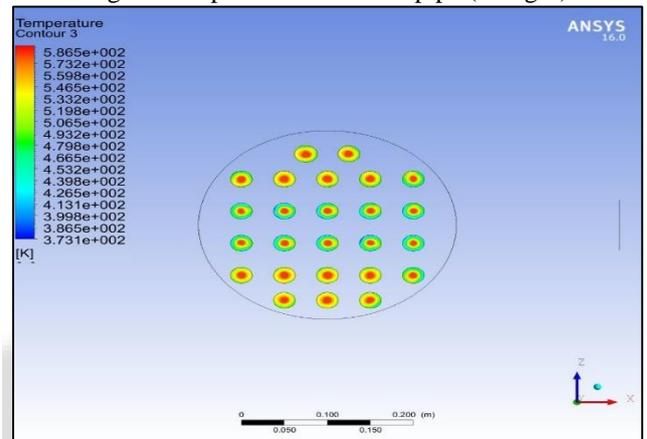
Fig. 8: Temperature at outlet of pipe (flue gas)
