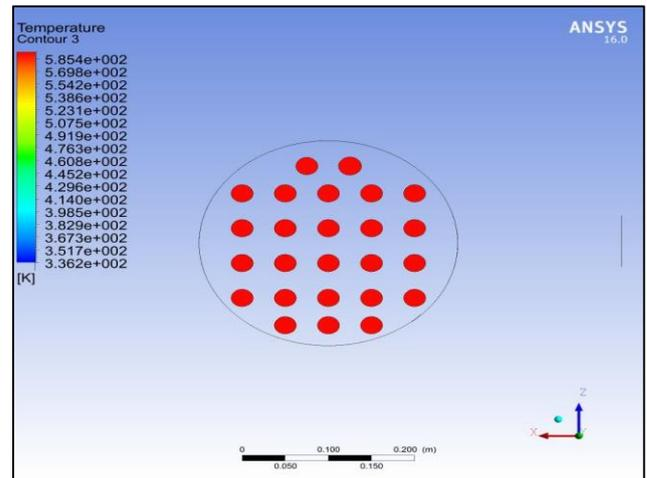
Fig. 7: Temperature at inlet of pipe (flue gas)
