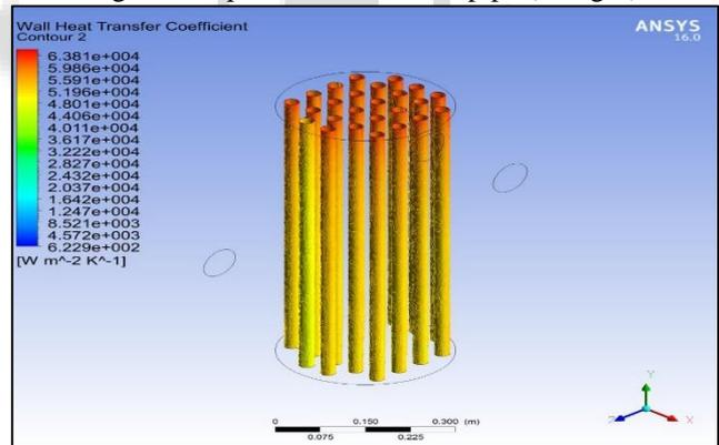
Fig. 9: Wall heat transfer coefficient along the tube
