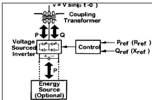
Fig. 1: Block diagram of Stat Synchronous Series Compensator
