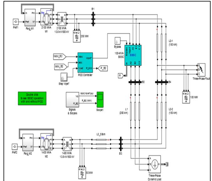
Fig. 4: Model of SSSC with POD
