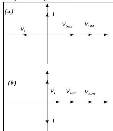
Fig. 2: Vector diagram of SSSC (a) Capacitive mode and (b) Inductive mode
