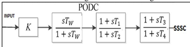
Fig. 3: Block diagram of POD
