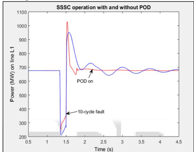
Fig. 8: fault analysis with and without SSSC-POD
