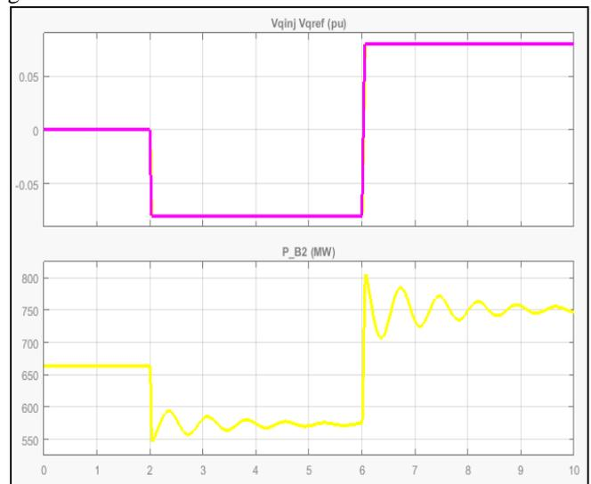
Fig. 5: SSSC inductive and capacitive mode POD OFF
