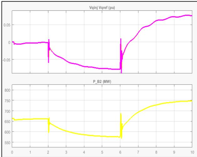
Fig. 6: SSSC inductive and capacitive mode POD ON
