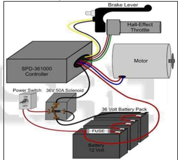
Fig. 2: Wiring sequence for the operation of Motor
