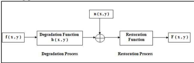
Figure (3.1) – Image Degradation and Image Restoration Process
