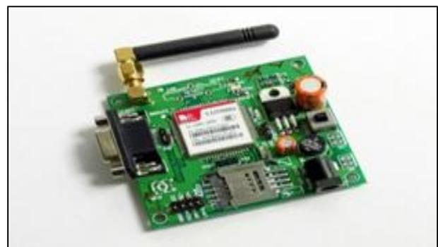
Fig. 5: GSM Modem
