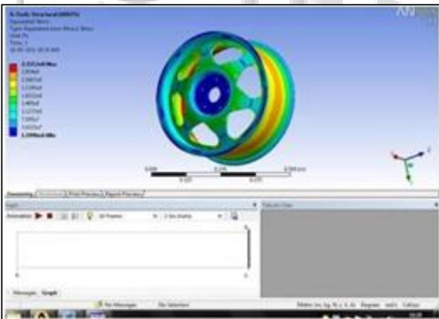
Fig. 3: Analysis of wheel Rim using ansys
