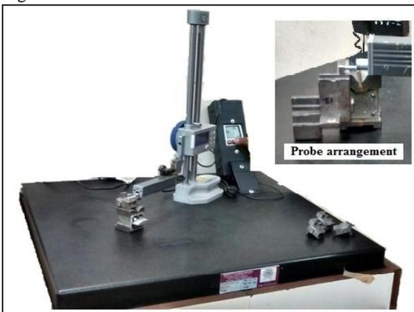
Fig. 2: Surface roughness measurement set-up and probe arrangement
