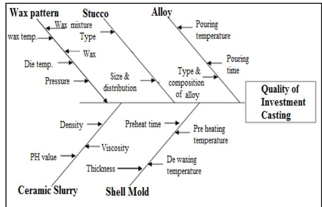
Fig. 1: Process parameters affecting Investment Casting process
