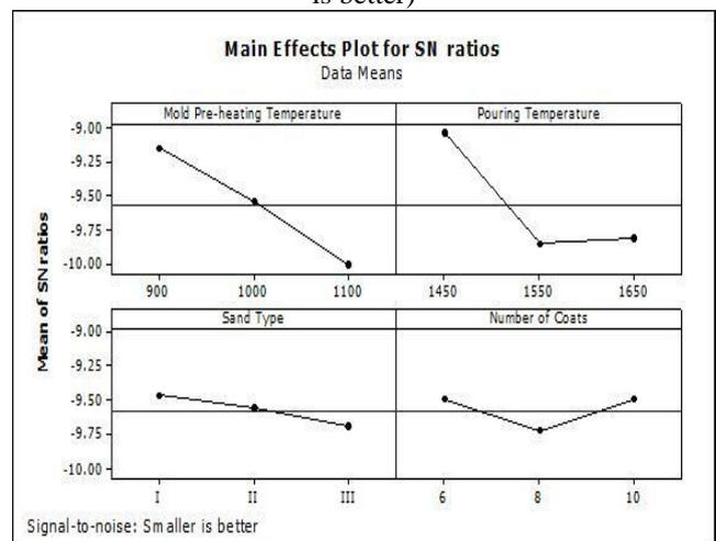
Fig. 3: Effects of process parameters on S/N ratio (main effects)
