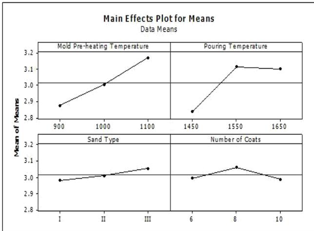
Fig. 4: Effects of process parameters on Surface Roughness (raw data) s
