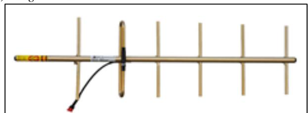
A Yagi antenna is a directional antenna consisting of a driven element such as dipole or folded dipole and additional parasitic elements, typically a reflector and one or more directors. It radiates in only one direction and is most commonly used in point-to-point communications.
