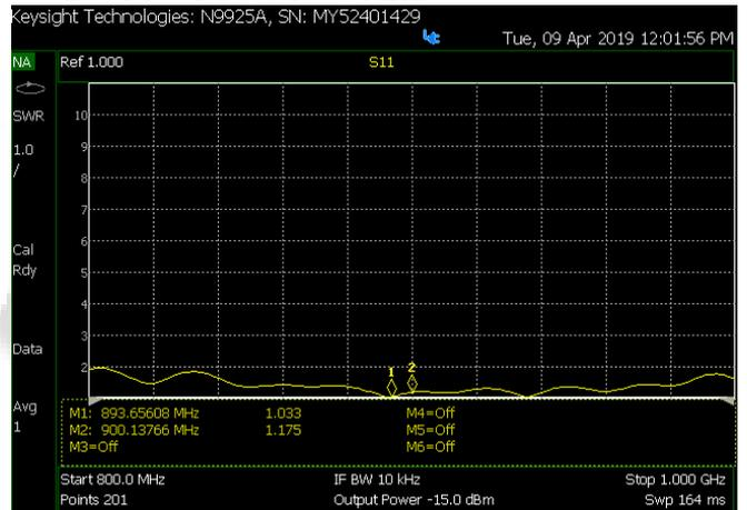
Fig: Simulation result – Monopole Antenna
