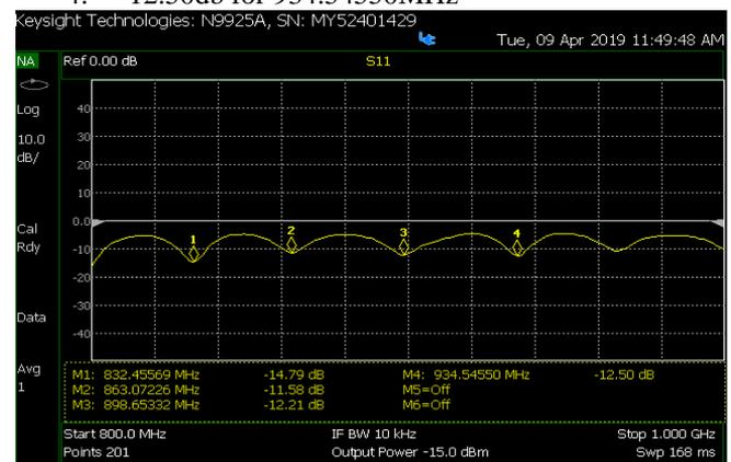
Fig: Simulation result – Yagi Uda Antenna (Log Chart obtained on Network Analyzer)
