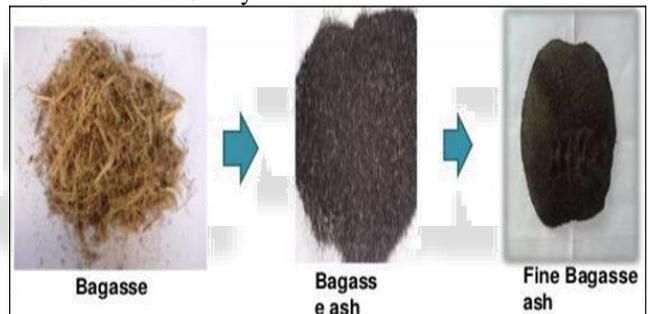
Fig. 1: Pictorial representation of Bagasse, Bagasse Ash and Fine Bagasse Ash
